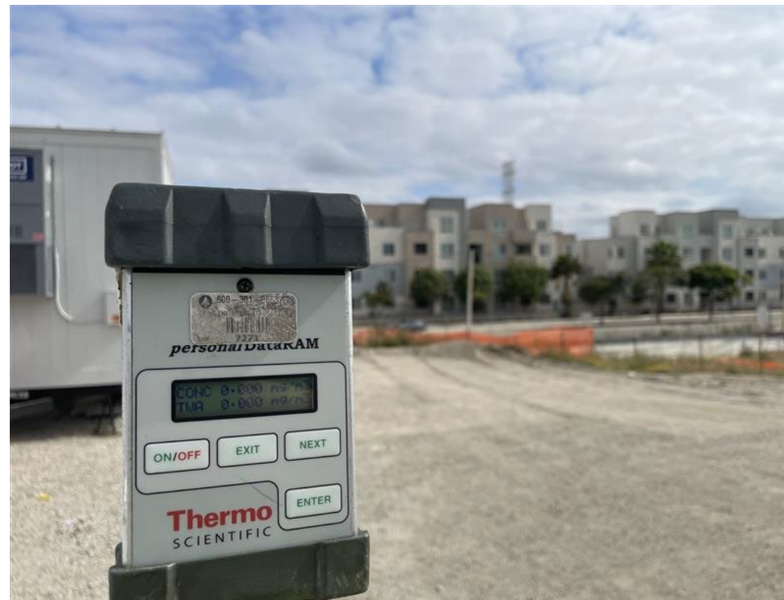
pDR-1000AN Measuring PM10 at Portable Perimeter Station 1 (PP-1)
