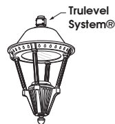
SIG18-P-AL Max Weight = 28 lbs Max EPA = 1.08 36 LED Max
