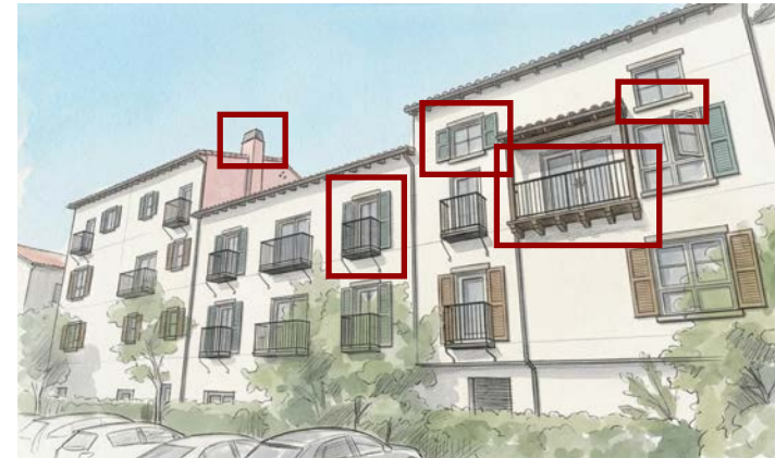
Architectural Projection Example: Pop-outs, balconies, window sills, shutter details, and chimneys pictured.
