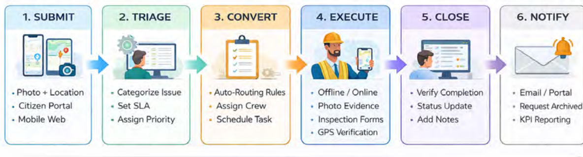
Figure 19: Closed-loop citizen service request workflow integrated with work orders, notifications, and analytics.
