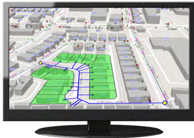
Figure 5: GeoViewer Valve Isolation Module
